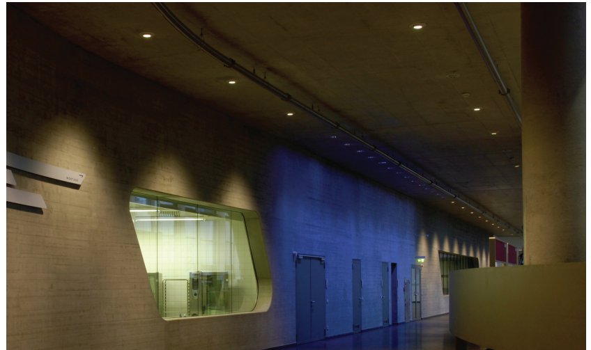
▲ Light is used here to add structure to the bare concrete surfaces: double-focus downlights illuminate these thoroughfares with precisely scalloped beams providing high visual comfort.
